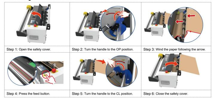
NOTE: Please ensure the kraft paper enters the feeding inlet with both sides flush. Incorrect feeding may cause machine jams or paper tearing.
