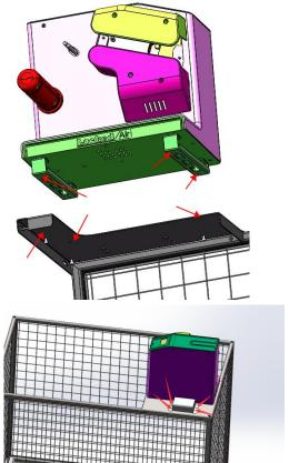
Step 7: Install the control box and sensor, the size of bolt isM5\*12, see picture;
