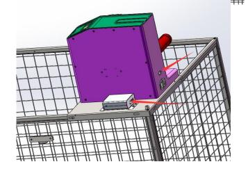
Step 10: Spare part installation, fix the feeding port, bolt size M6\*50, fixing the brusher, bolt size M6\*30, see picture;
