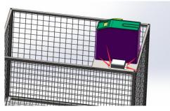
Step 8: Fix the stand of sensor, clamp with clip, bolt size M6\*12, to make sure two sensors are in the same line, see picture;
