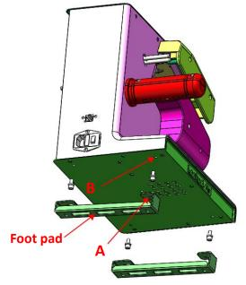
Align the hole of foot pad and hole Step 6: on the cart:
